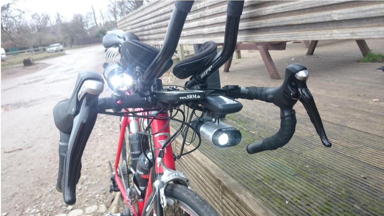
I was using this “bike” on the turbo in 2018. I put road bars on it with road shifters so that I could change the extensions easily with the cabled 105 mechs.
